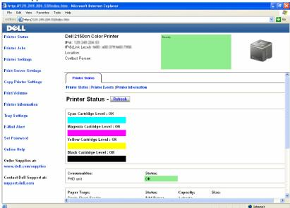
To fill out printer inventory reports requiring the asset tag number of all the printers in your area, use the Printer Information feature in the Dell Printer **Configuration Web Tool**. Enter the IP address of each printer on the network to display the asset tag number.
